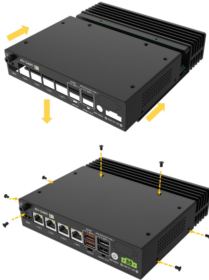
Figure 3-6: Back Cover Installation
