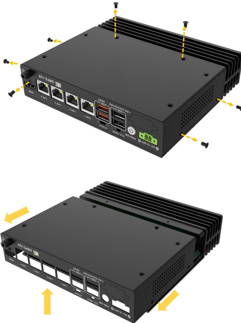
Figure 3-1: Remove the Cover
