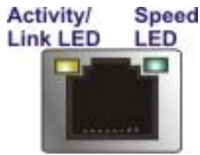
Figure 3-11: RJ-45 Ethernet Connector
